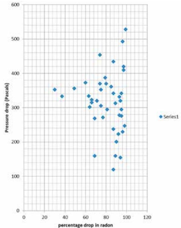
**Figure 3** Comparison of pressure drop & % drop in radon.
