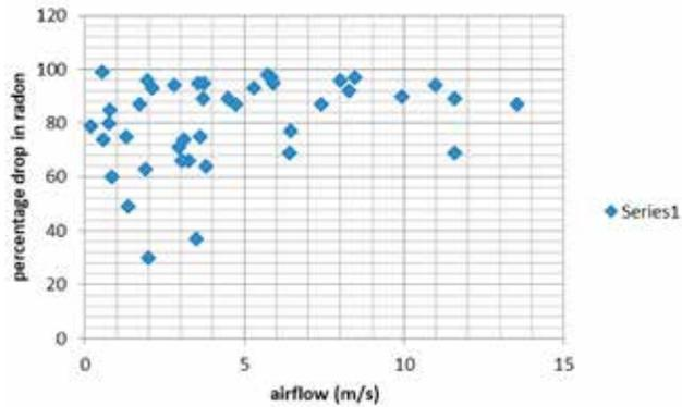
**Figure 4** Comparison of airflow & % radon reduction.
