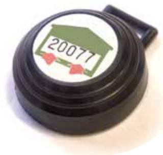
**?** Bqm<sup>-3</sup> = Becquerels per cubic metre, the concentration of radon in the air.
